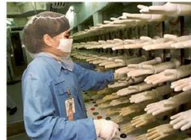
An employee strips latex gloves off their molds inside a stripping-booth at a plant in Penang, Malaysia March 12, 1996. Credit: AP Photo/Mike Elze
